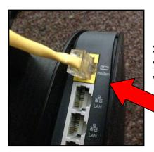
2. Use Ethernet cord to connect to port, then connect the other end to your computer or your router. If you are connecting to the router, you will need to connect to the port labeled "modem" or "switch."
